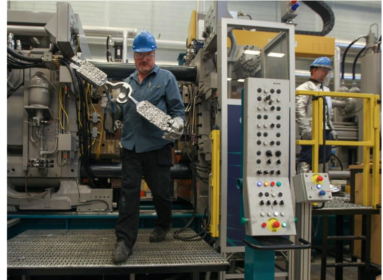
Canmet MATERIALS A national laboratory of Natural Resources Canada, Hamilton, ON 1200t HPDC machine
